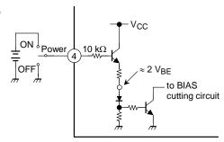
Figure 2 With Pin 6 Set to High, Power is Turned ON
